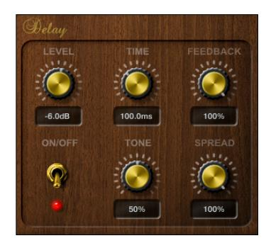
*Spread*: sets the stereo image of the repetitions generated by the delay, where 0% is mono, and 100% is full stereo for a ping-pong delay effect.
